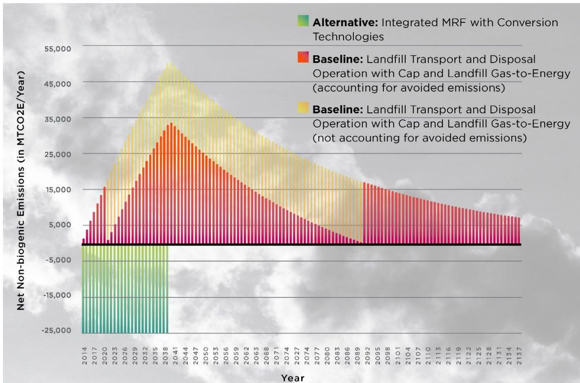
The analysis results found that the Baseline Scenario (landfill disposal with LFG-to-energy of 1000 tpd of MRF residuals) generates 2.31 million more MTCO<sub>2</sub>E of net GHG emissions than the Alternative Scenario (Integrated MRF with Conversion Technologies).
