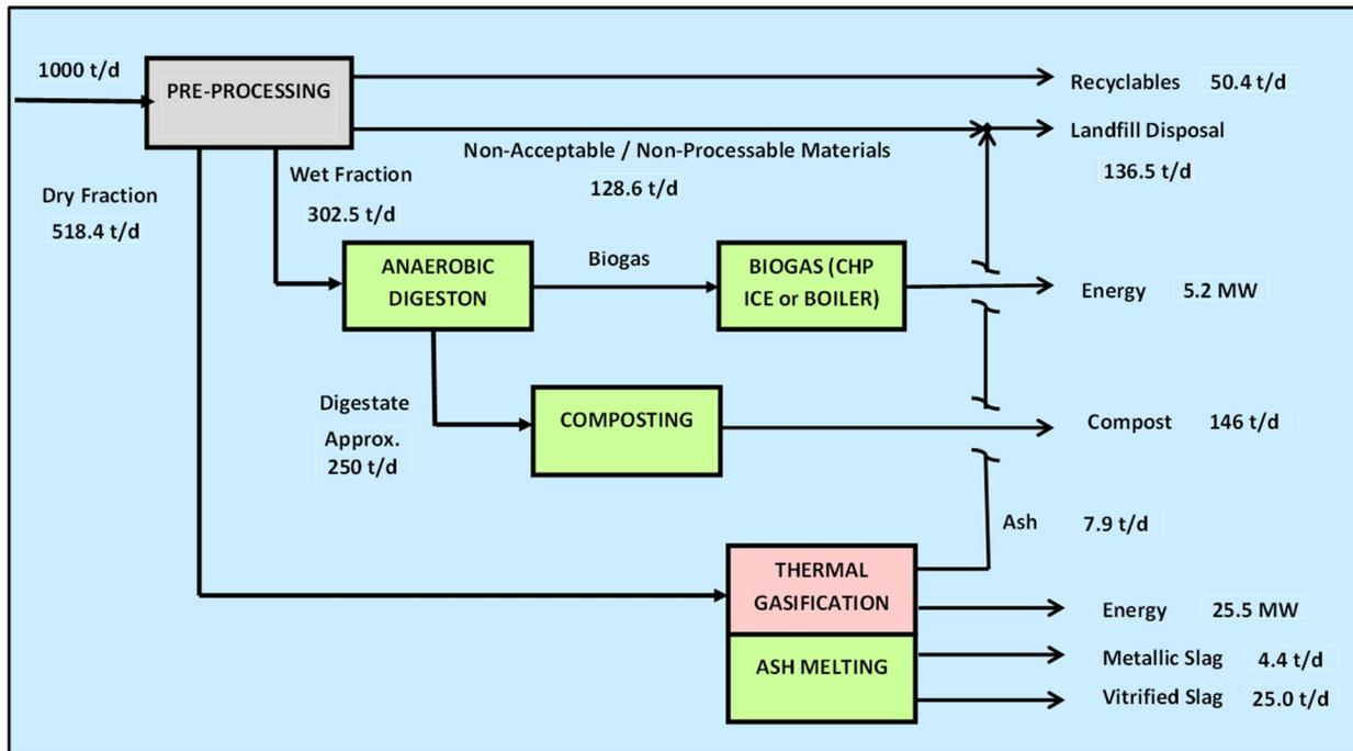
Note: Mass balance presents general mass flow of tons of mixed waste MRF residuals material into system and resulting tonnage to disposal, recyclables, compost and slag. Mass Balance does not show input tons of coke, process water, chemicals, supplemental chemicals for emissions control and control of viscosity of slag, etc.
