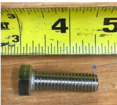
1.5 inch threaded bolt of truss splice
