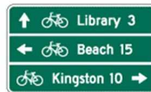
Bicycle guide signs are green, and can include destination, direction and distance information. (MUTCD sign D1-3C).
