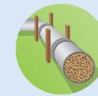
Slurry pipelines are used in conjunction with the dredging sediment removal alternative, and involve the pressurized mixture of water and sediment dredged from a reservoir.
