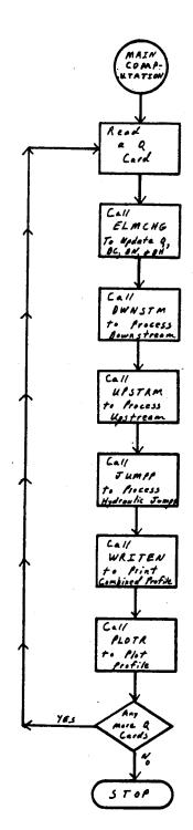
Controls the Computation of the Water Surface Profile.
