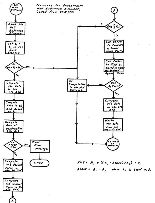
Processes the Downstream Wall Exit Element, Called from DWNSTM
