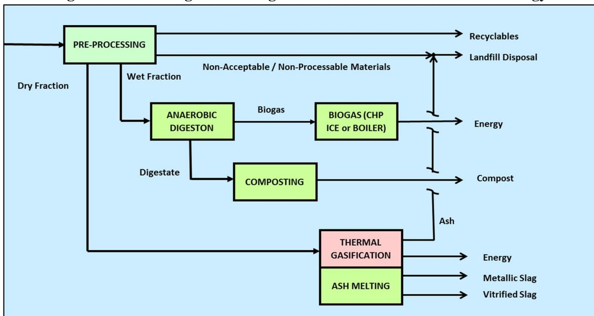
Note: The boundary of the analysis did not include transport of heat sources (coke) for thermal gasification or compost and slag to off-site receiving facilities
