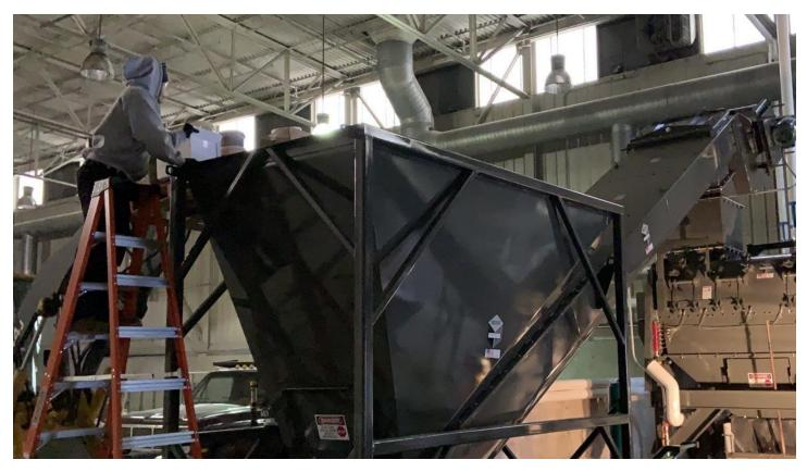
The old Recycling Center – now the Muscatine Organics Recycling Center – is using Scott Equipment T42 Turbo Separator to help them separate food waste from plastic packaging. The organic waste is used to create fertilizer and renewable natural gas.
