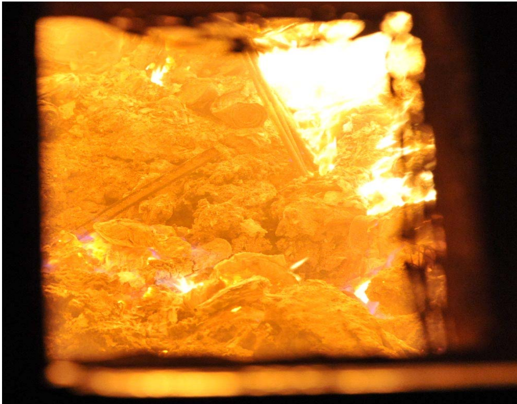
Figure 9. Combustion on the Grate of SERRF Incinerator (UCLA Engineering Extension)
