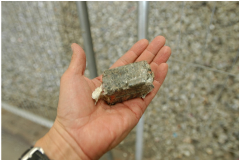
Figure 42. "Cube" form of RDF-5 (UCLA Engineering Extension Photo)
