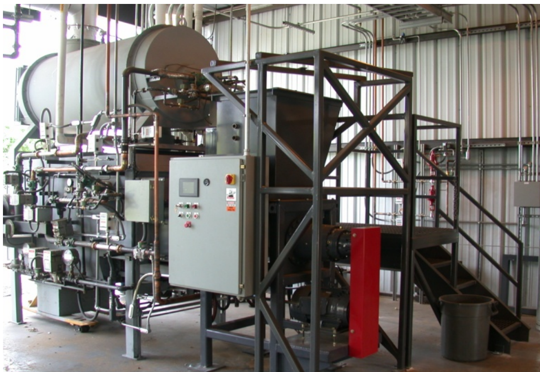
Figure 25. BRI/INEOS Two-Stage Stepped Hearth Gasifier (Fayetteville, Arkansas)
