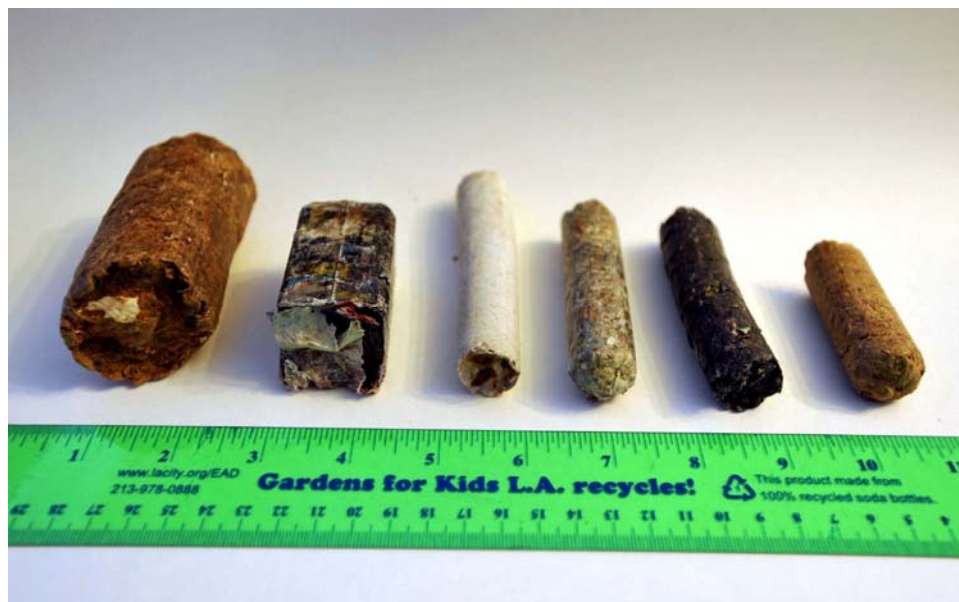
Figure 44. End view of various forms of "densified RDF" RDF-5 (UCLA Engineering Extension Photo)
