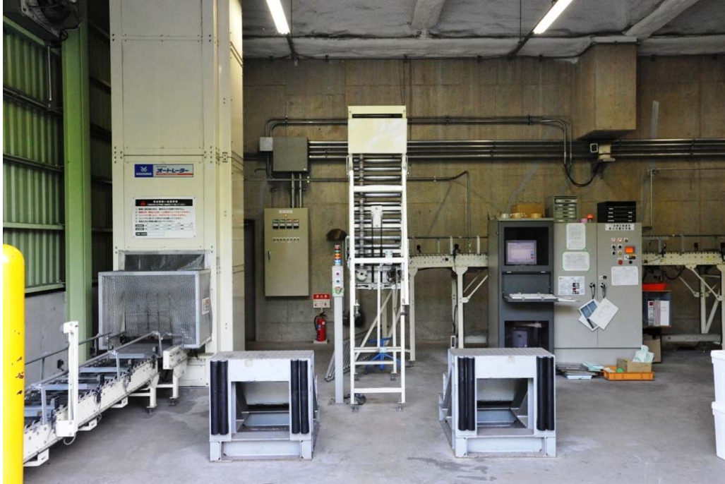
Figure 47. Eco-Frontier Kasama-City, Japan, MSW Gasification Facility, medical Waste Receiving and Unloading Section (Courtesy of JFE Engineering)
