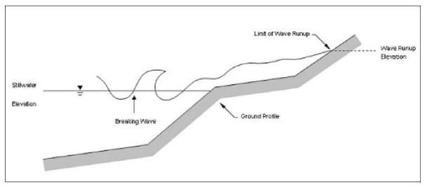
Figure 5: Wave Runup Transect Schematic
