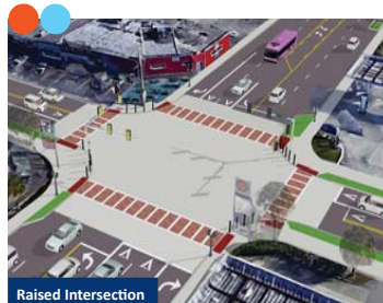
Raised Intersection Raised Intersections reinforce slow speeds and encourage motorists to yield to pedestrians in the crosswalk.
