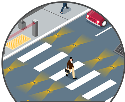
EMBEDDED CROSSWALK LIGHTS
