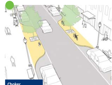
Choker Chokers are two curb extensions on opposite sides of the street that encourage drivers to slow down by making the street narrower. They can also be used as part of mid-block pedestrian crossings.
