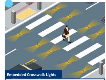
Embedded Crosswalk Lights
