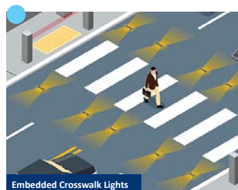
Embedded Crosswalk Lights Embedded crosswalk lights provide clear visibility and enhance the driver's ability to spot pedestrians. To achieve this, the luminaires must be strategically positioned to minimize any silhouette effect on the pedestrian and ensure positive contrast for better visual identification.
