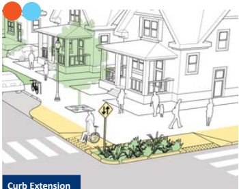
Curb Extension Curb extensions narrow the roadway and reduce the crossing distance and allow pedestrians and drivers to see each other when parked vehicles would otherwise block visibility.
