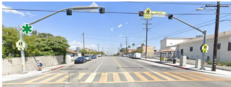
* Pedestrian-activated warning beacon at a continental crosswalk East Los Angeles, LA County UA (Source: StreetView)
