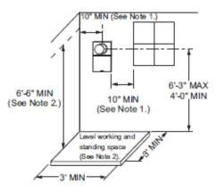
Surface-Mounted or Semi-Flush Meter Installation
