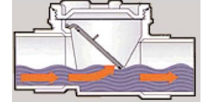
Properly installed backwater valve allows household waste waters to flow to the sewers.
