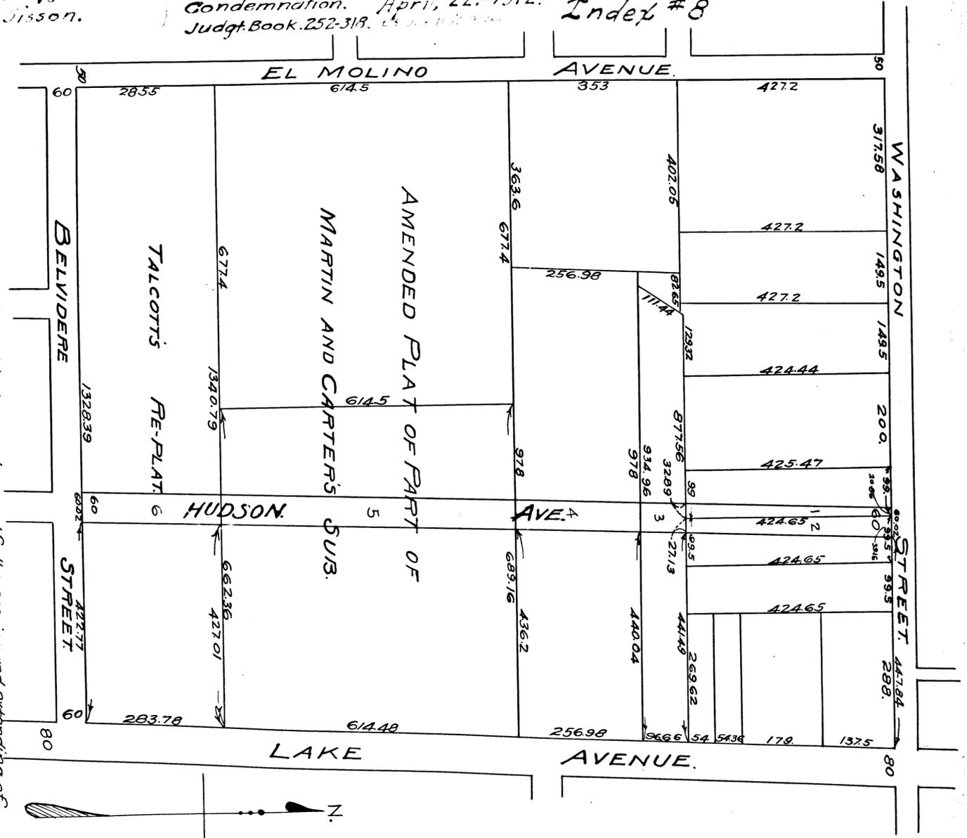
Map showing land sought to be condemned for the opening and extending of HUDSON AVENUE, from Belvidere Street to Washington Street, Pasadena, Cal. Note: Shaded portion shows land sought to be condemned. Scale: 1"=200'
