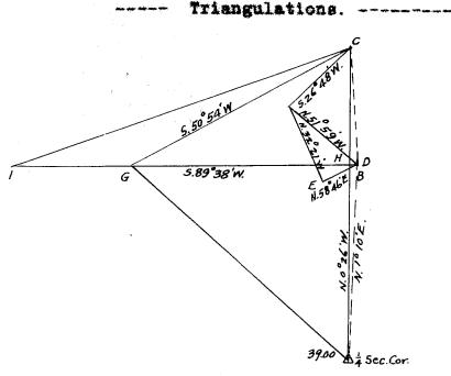
At B, I turn off the brg. N.58°46' E.in which marked point "D"; and reversed the brg. B. 58°46' W. in which marked point "E"; repeated the measure of the line DE and find it 5.17 dks. long for a base.
