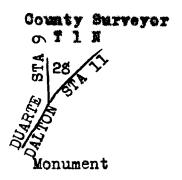
This corner was recestablished by the County Surveyor of Les Angeles County at a point determined by proportion bet. Cor. No.10 and Cor. No. 12 of Rancho Asusa Dalton and on a bearing from Cor. No. 10 determined from a number of iron pipes and pins/at irregular intervals along the line that have been accepted and used as marking this property line for many years.
