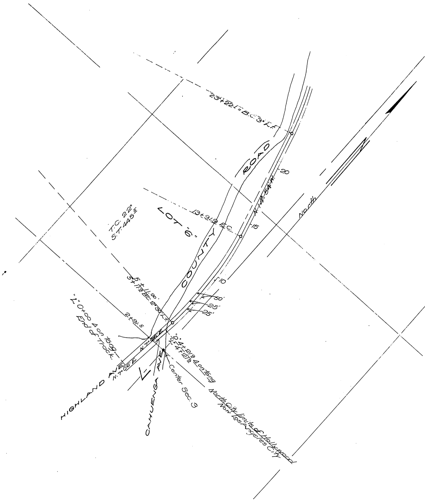
Plat Showing location of L AND D LINE for proposed Railway from Hollywood to Lanckershim in the
