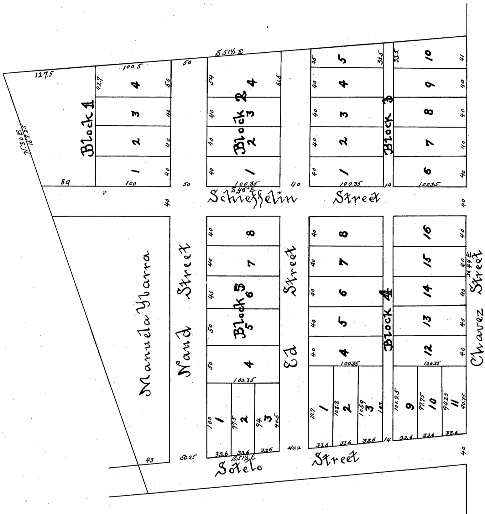
Schieffelin Tract in Los Angeles City, California Surveyed April 1883 by Hansen & Solano Magnetic Courses = Scale 40 ft per inch
