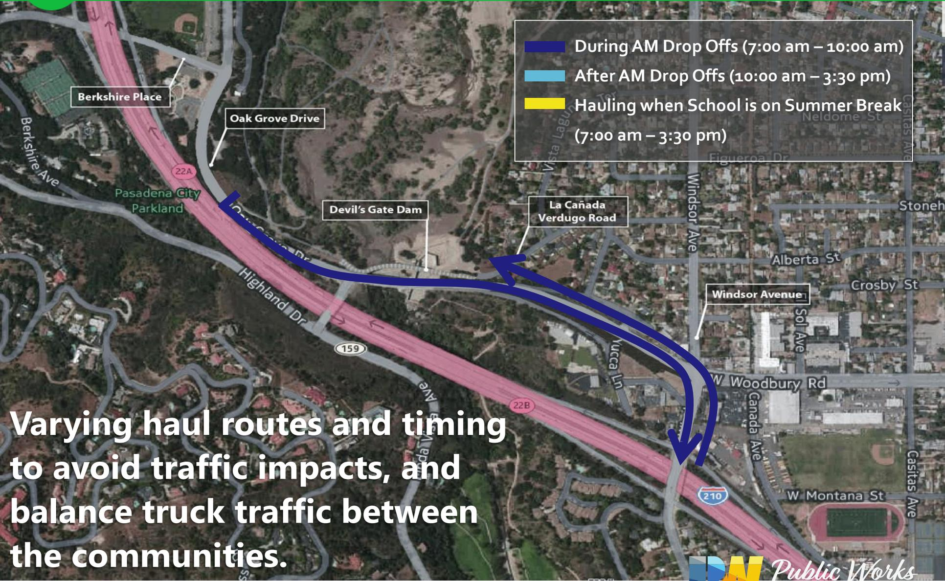
Varying haul routes and timing to avoid traffic impacts, and balance truck traffic between the communities.
