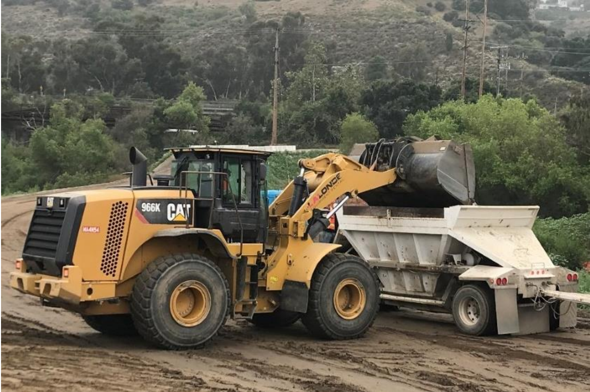
6/27/19 – Loader patting down tops of load to ensure freeboard compliance.
