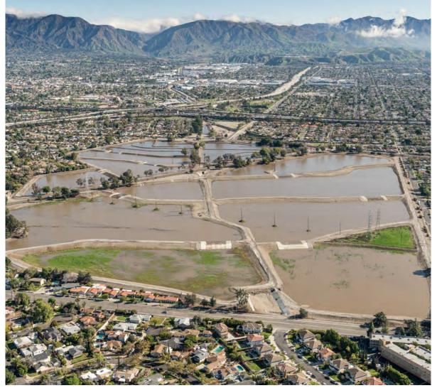
Figure 71. Our local groundwater basins are recharged using different techniques, such as spreading grounds like this one in Pacoima. Source: LA County Public Works, 2018.
