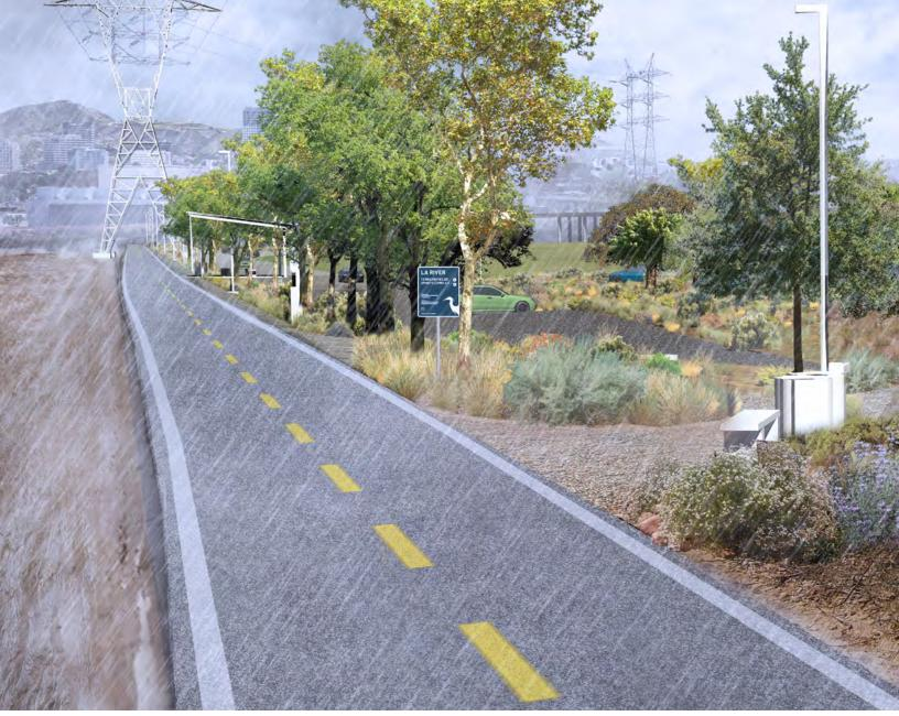
Figure 317. During flood events, the Ferraro Side Channel could play an infrastructural role, transporting water downstream around this area of higher flood risk.
