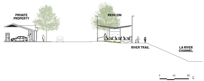
Figure 308. A small grade separation provides a buffer between the bike path and the pavilion.
