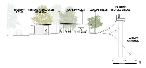
Figure 309. A section through the landside gathering pavilion shows how the buildings shield the bike path and courtyard space from an adjacent highway on-ramp.
