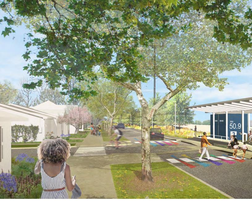
Figure 307. A street terminating at the river's edge is a typical upper river condition in the San Fernando Valley. This design example captures and treats local stormwater flow before it enters the river while also providing access and amenities to the adjacent community.
