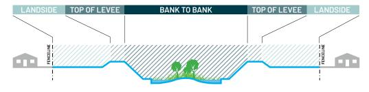
Figure 19. There are a few trapezoidal channel typologies along the LA River. The trapezoidal channel either has a soft or concrete bottom and may or may not have visible levees.
