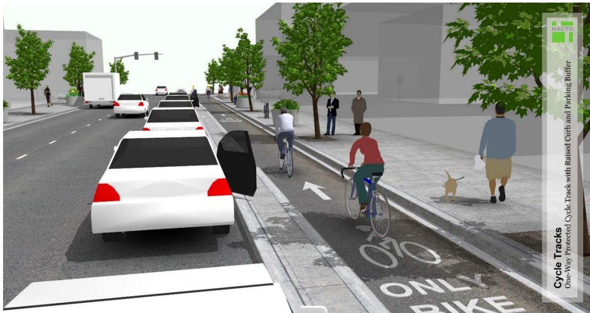
Figure 7-2. On-street parking may be used to separate a Class IV bikeway from vehicle traffic
