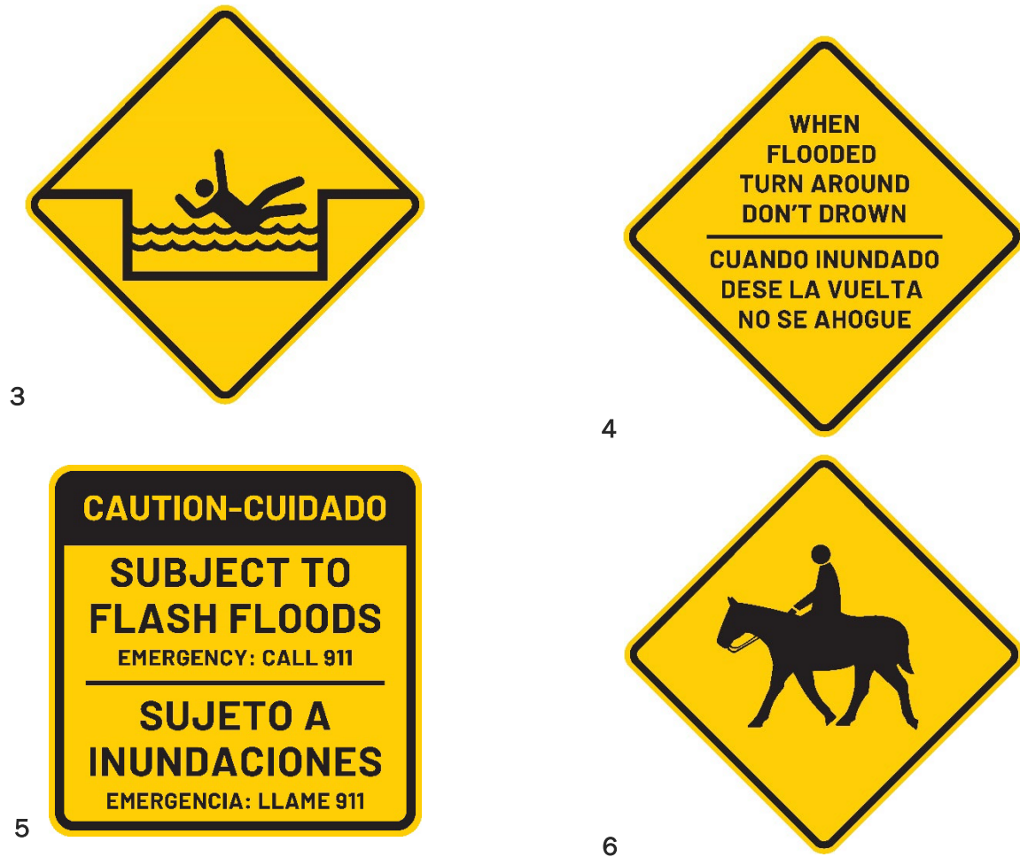
Figure 8-17. The signs shown above (3-6) are examples of warning and safety regulations signs that are standard designs and must not be altered. These guidelines do not provide artwork for these standard signs. Designers should consult latest MUTCD guidelines.
