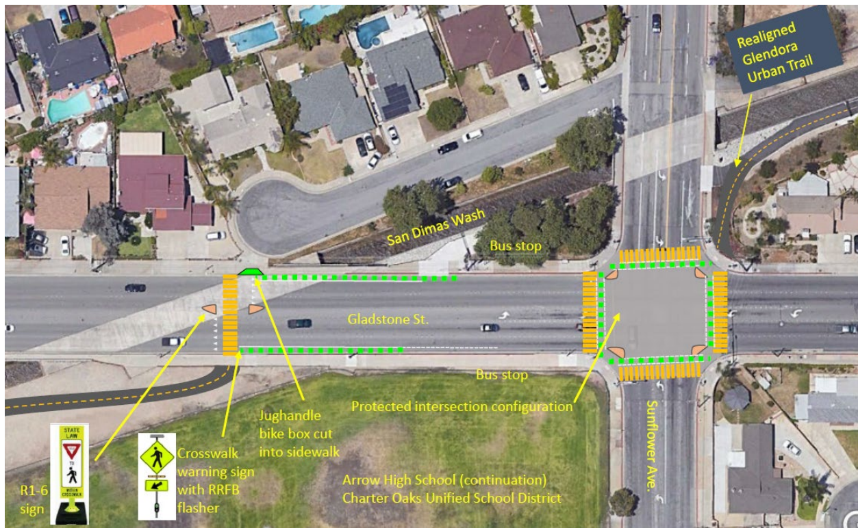
Figure 9-3. Hypothetical greenway crossing treatment near a signalized intersection
