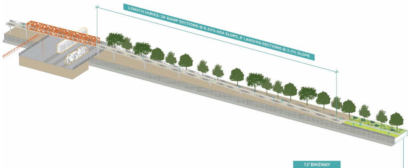
Figure 4-16. Overcrossing diagram with clearance and ADA slope
