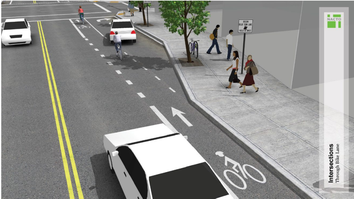
Figure 5-8. Example of a bike lane at an intersection with a right-turn-only lane
