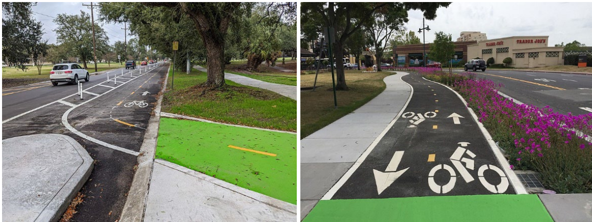
Figure 7-5. Examples of flexible post (left) and landscape island (right) separators
