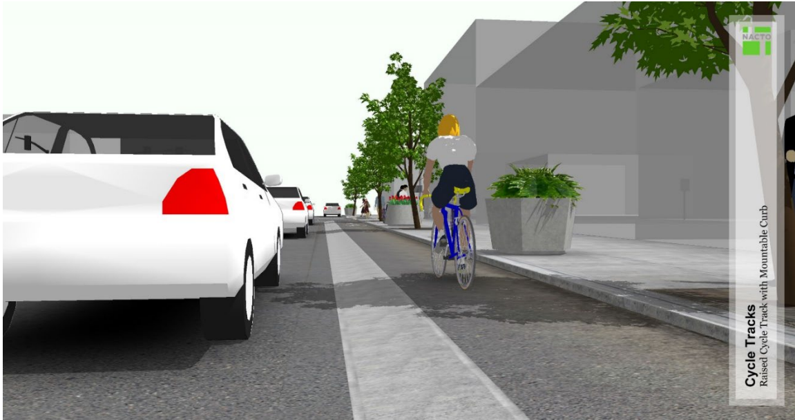
Figure 7-7. Class IV bikeway example
