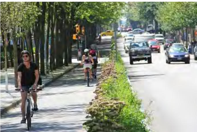
Figure 1-8. Example of an inflexible barrier separating bikeway from traffic (Class IV bikeway)
