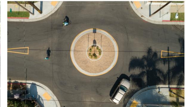
A **traffic circle** is a raised island located in the center of an intersection around which traffic must circulate. They may be used to lower vehicle speeds and conflicts at the intersection of two roadways. They are typically operated as two-way or all-way stop-controlled intersections
