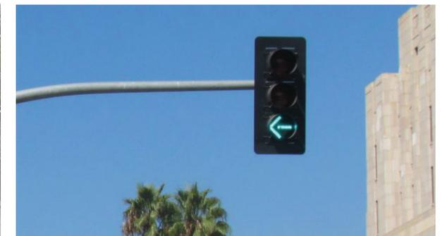
**Left Turn Signal Phasing** provides a green arrow for left turning vehicles while stopping conflicting vehicles and pedestrians.
