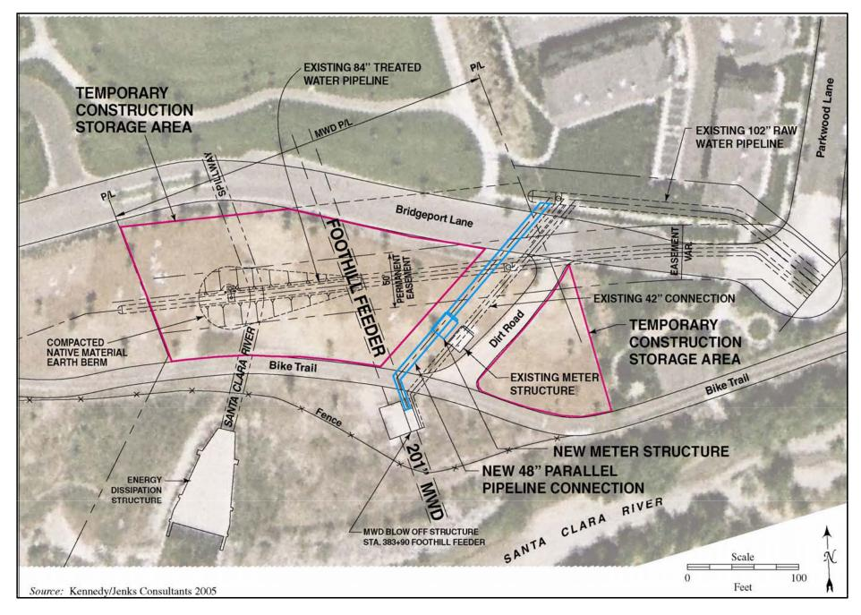
CLWA-8.2 Foothill Feeder Connection (CLWA-8) Detail of Connection
