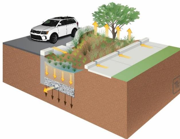
Figure B-2-6. Typical distributed bioretention and biofiltration schematic showing underdrain option (arrows indicate water pathways).
