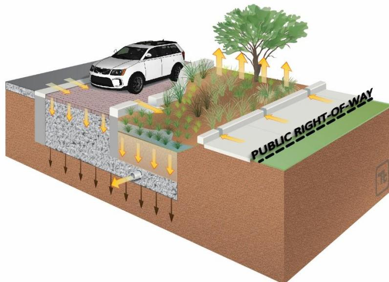
Figure B-2-8. Typical distributed green street schematic (arrows indicate water pathways).
