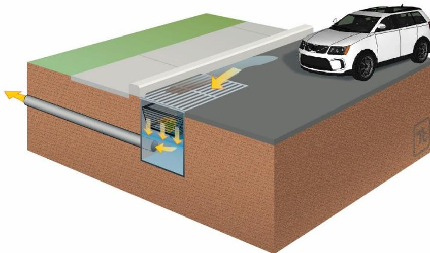
Figure B-2-13. Typical distributed source control structural BMP (arrows indicate water pathways).
