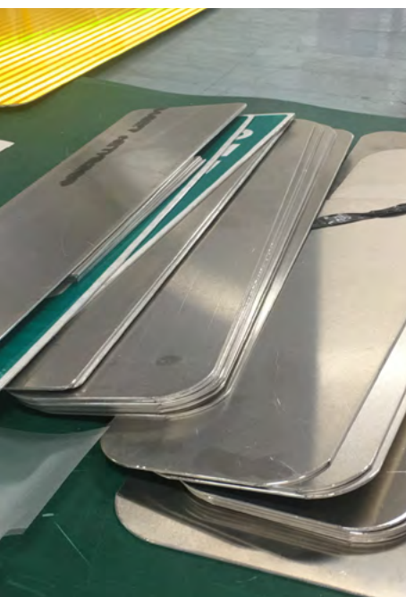
Figure 115. Aluminum with rounded corners is used as the base of many types of signs. Source: OLIN, 2019.
