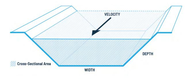
Figure 6. Open Channel Diagram. Shown here is a stylized section of an open channel representing that total flowrate is a function of velocity multiplied by cross-sectional area.
