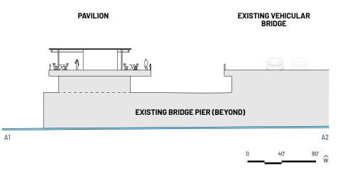
Figure 301. A section through the Los Feliz Bridge shows how an additional pedestrian river crossing created on the existing bridge piers.
