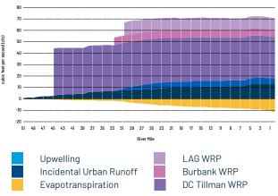
Figure 284. These are the current (2020) dry weather flows by river mile along the LA River. Source: Adapted from OneWater LA 2040 Plan. 2018.
