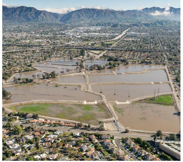
Figure 66. Our local groundwater basins are recharged using different techniques, such as spreading grounds like this one in Pacoima. Source: LA County Public Works, 2018.
