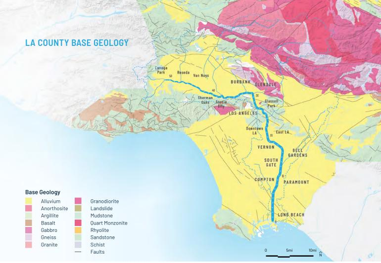
Figure 34. LA County Base Geology. The LA River geology is alluvium and can be over 20,000 feet deep in places. Source: California Geologic Map Data, USGS, 2005.
