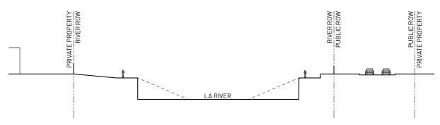
Figure 260. Converting an existing trapezoidal channel into a rectangular channel can result in a substantial increase in channel capacity; however, this strategy should always be combined with other multi-benefit components.
