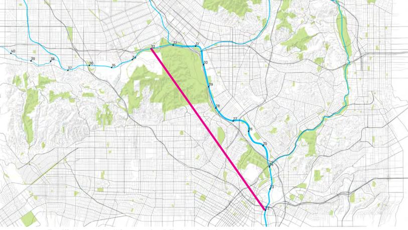
Figure 267. A bypass tunnel would divert water at river mile 33 and return it to the river at river mile 22.
