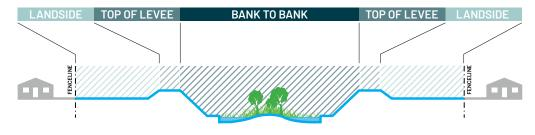
Figure 16. There are a few trapezoidal channel typologies along the LA River. The trapezoidal channel either has a soft or concrete bottom and may or may not have visible levees.
