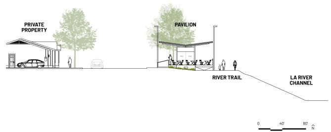
Figure 297. A small grade separation provides a buffer between the bike path and the pavilion.
