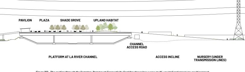
Figure 312. The section through the Compton-Paramount Connectivity Corridor shows how a new multi-use trail and greenway could connect across the LA River and 710 Freeway which stitching together a variety of program and habitat areas.
