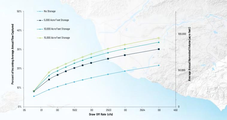
Figure 280. With storage and variable diversion rates, the LA River can reliably provide upwards of 50,000 acre-feet per year of treated water for groundwater recharge.
