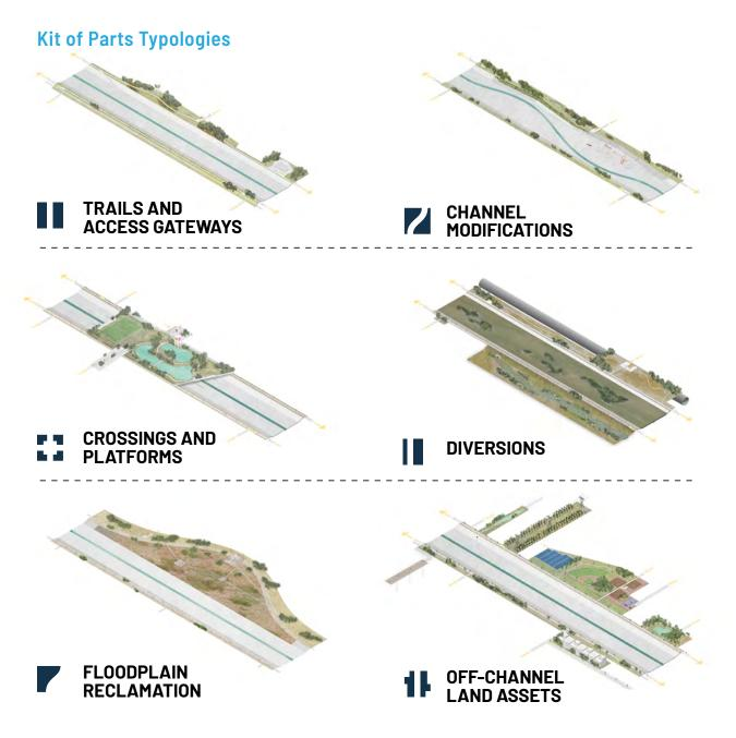
Figure 215. Kit of parts design components can be categorized into six infrastructure and urban river typologies. These drawings illustrate a selection of these components applied to a typical trapezoidal channel.
