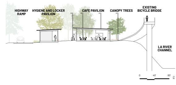
Figure 299. A section through the landside gathering pavilion shows how the buildings shield bike path and courtyard space from adjacent highway on-ramp.
