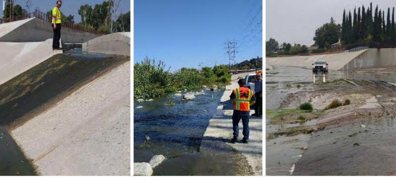
Figure 355. Outfall, soft bottom vegetation, river bottom inspection. Source: Geosyntec, 2018.
