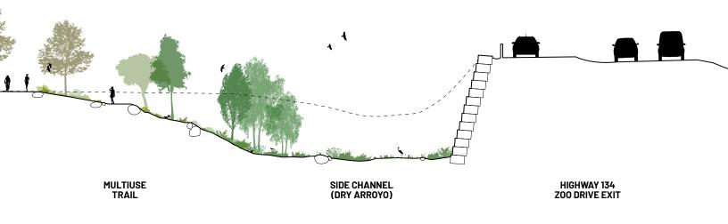
Figure 304. The section shows how a new side channel could be created on underutilized land between the site's existing athletic fields and the 134 Freeway.
