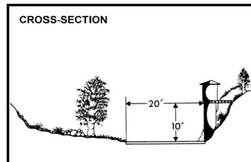
**RECORDER** - Continuous water stage.**METHOD OF MEASUREMENT** - Wading**DRAINAGE AREA** - 11.2square miles.**LOCATION** - 1,000 feet above Little Creek and 4.5 miles south of Little Rock.**REGULATION** - None.**DIVERSION** - None.**CHANNEL** - Sand, gravel and boulders.**CONTROL** - Concrete and rubble wall.**LENGTH OF RECORD** - September 29, 1953 to date.**REMARKS** - No high flow measurements.
