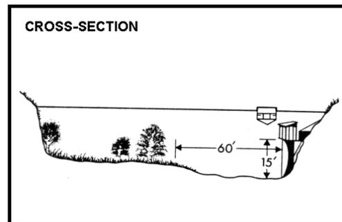
**RECORDER** - Continuous water stage.**METHOD OF MEASUREMENT** - Stream gaging.**DRAINAGE AREA** - 49.2 square miles.**LOCATION** - 2.0 miles above Little Rock Dam, 5.0 miles south of Little Rock.**REGULATION** - None.**DIVERSION** - None.**CHANNEL** - Sand, gravel, and boulder, natural in section.**CONTROL** - Channel forms control.**LENGTH OF RECORD** - October 1, 1930 to date.**REMARKS**
