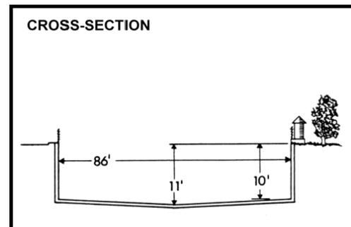
**RECORDER** - Continuous water stage.**METHOD OF MEASUREMENT** - Wading or from Concord Street bridge.**DRAINAGE AREA** - 26.8square miles.**LOCATION** - 800 feet east of San Fernando Road, 2.0 miles northwest of Glendale.**REGULATION** - Partially regulated by several debris basins.**DIVERSION** - None.**CHANNEL** - Concrete, rectangular section.**CONTROL** - Channel forms control.**LENGTH OF RECORD** - December 2, 1935 to date.**REMARKS**
