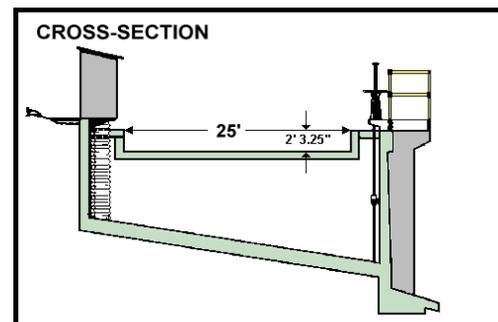
**RECORDER** - 5 min. interval data logger.**METHOD OF MEASUREMENT** - Weir formula with gage height observation.**DRAINAGE AREA** - 202.7square miles.**LOCATION** - On the concrete conduit which diverts from San Gabriel Dam, 160 feet below the dam.**REGULATION** - Regulated in section.**DIVERSION** - None.**CHANNEL** - 25 foot concrete weir.**CONTROL** - Channel forms control.**LENGTH OF RECORD** - February 26, 1933 to date.**REMARKS** - Approximate capacity 95 second-feet.
